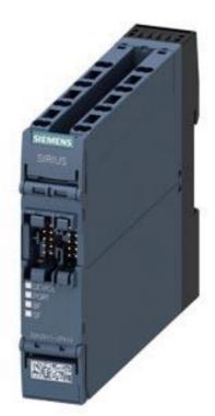
SIRIUS, interface module PROFINET interface for safety relay 3SK2 as of E05 and 3RK31 as of E04 PROFINET IO interface 100 Mbit/s, RJ45 22.5 mm width Spring-type terminal Can be parameterized via Safety ES without connecting cable
