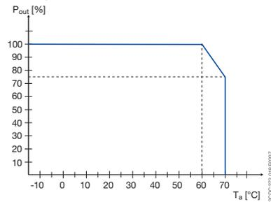
Characteristic curve of temperature at  $U_{out}$
