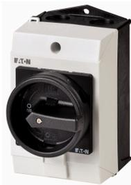
**Main switch, 3 pole + 2 N/O + 1 N/C, 20 A, STOP function, 90 °, Lockable in the 0 (Off) position, surface mounting**
