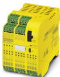
Freely configurable safety module with 20 safe inputs and 4 safe outputs; 4 alarm, 2 clock, and 2 ground switching outputs; diagnostics possible via bus gateways, up to SILCL 3, Cat.4/PL e, SIL 3, EN 50156, plug-in screw connection terminal blocks
