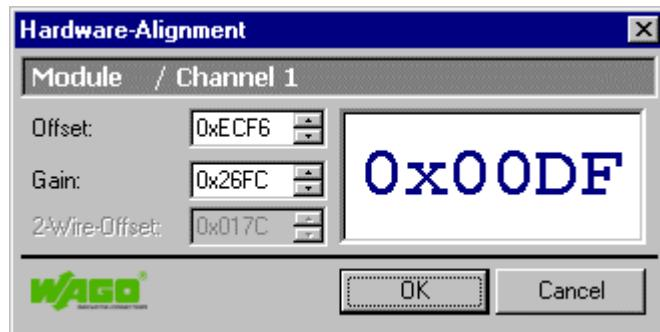
Use the edit boxes **Offset** and **Gain** to change the offset and gain values for the hardware alignment. If required, you can adjust the offset for the wire resistance with the edit box **2-Wire Offset** when performing a 2-wire measurement. Inputs are done in hexadecimal format.
