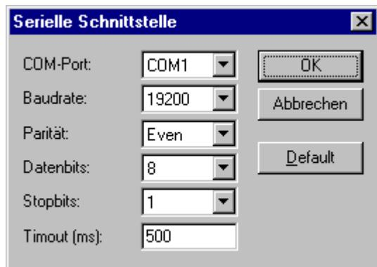
Select the serial PC interface for communication with the coupler. All other settings (baud rate, data bits,...) are fixed to default values for communication with the **WAGO-I/O-SYSTEM 750** and not changeable. The dropdown list shows all available COM-ports, which are not occupied by other applications.
