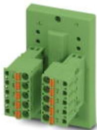
The VARIOFACE feed-through module implements a 1:1 connection between plug-in push-in spring-cage connection terminal blocks and a D-SUB miniature socket strip (number of positions: 9). A separate ground tap is available.
