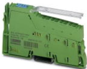
Inline digital input terminal, version for extreme conditions, complete with accessories (connector plug and labeling field), 8 inputs, 24 V DC, 1-wire connection technology
