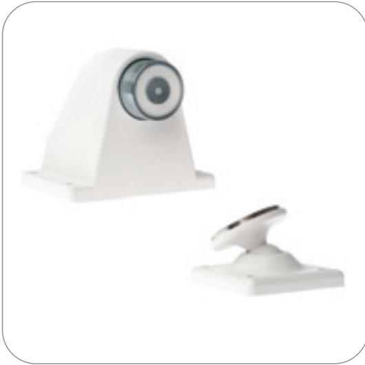
The DRX door retainer is ideally suited to applications where maximum protection is needed against vandalism or accidental damage. It features a rugged cast aluminium housing, a holding magnet with integral ejection pin and a manual release switch.
