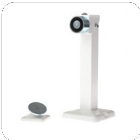
The DRP door retainers are available in both 500N and 1000N versions and also come in two standard lengths which can also be cut to length if required. The magnet is fixed within an adjustable head which allows the door retainer to transform between floor, wall or ceiling mounted. The stand and adjustable head are fabricated from steel providing a very robust structure. A moulded cover is included to conceal the mounting fixings once installed.
