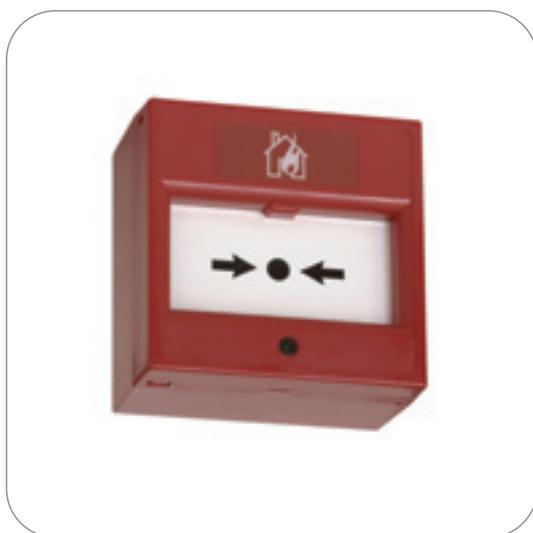
The EN54 approved call point has been designed to satisfy the EN54 requirements for approved fire systems. Supplied with break glass only which offers a protected plastic film covering to avoid stray glass fragments when the unit is activated.
