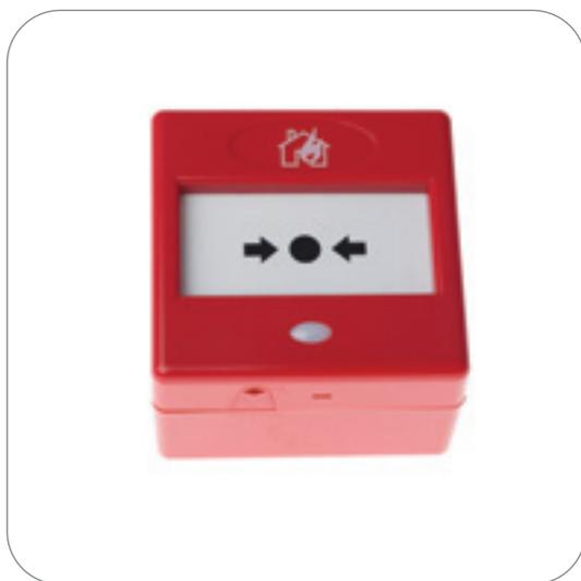
The EN54 compliant call point features a high intensity LED indicator and is supplied ready fitted with 470 Ohm, 680 Ohm resistors and a protective diode for use in most fire alarm systems. The unit comes supplied with the facility to choose either resettable or break glass operation as standard, making this unit the ideal choice.
