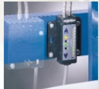
Choice of red, green, white or blue visible sensing beam. Choose from four sensing beam colors to optimize your R55F sensor for maximum sensitivity to any color. R55F sensors respond to light or dark signals to accurately detect even the most challenging color mark combinations, including 20% yellow on newsprint!
