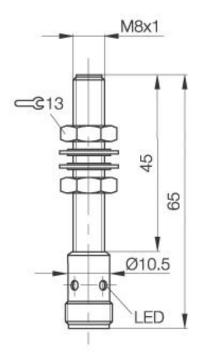
Inductive Sensors BES M08MH1-PSC20B-S04G M 8 x 65 normally-open Sn=2mm shielded
