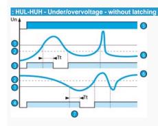
In overvoltage mode, if the controlled voltage exceeds the preset threshold for longer than the time set on the front face (0.1 to 3 s), the output relay opens and LED R is extinguished. During the time delay, this LED flashes.
