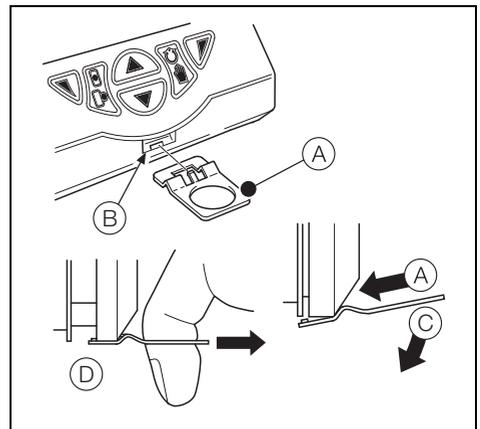
Fig. 4.6 Removing the Controller from its Case
