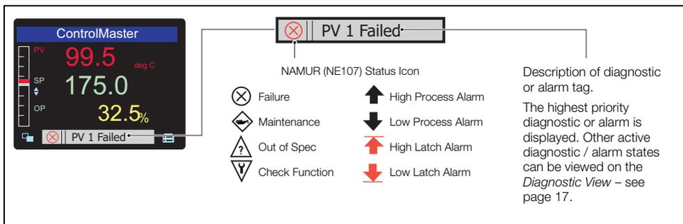
Fig. 5.1 ControlMaster Diagnostic Status Bar (ControlMaster CM30 Shown)
