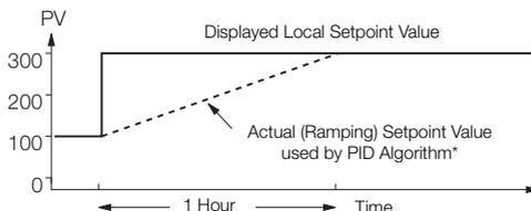
\*Example: Ramp Rate = 200 Increments / Hour
