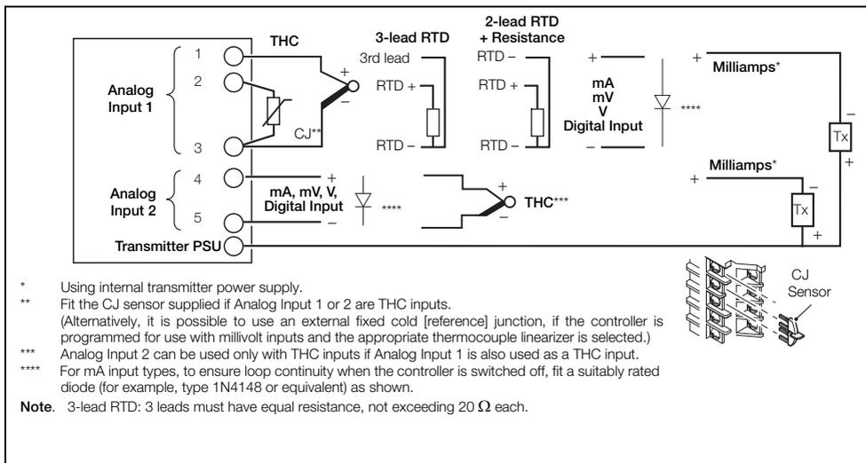
Fig. 4.10 Standard Analog Inputs (1 and 2)
