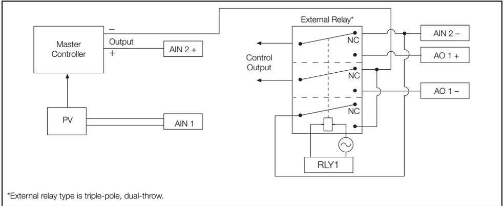
Fig. 8.1 Parallel Connection
