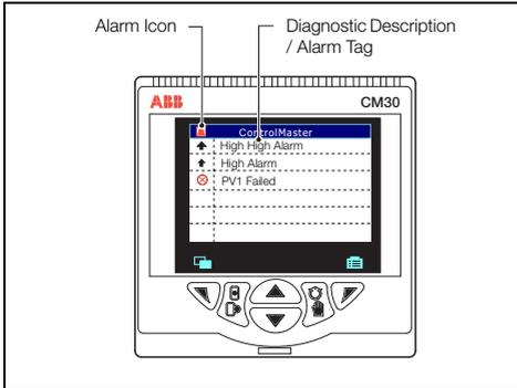
Fig. 5.2 ControlMaster Diagnostic View (ControlMaster CM30 Shown)
