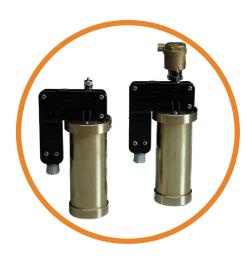
The switch is based on a simple principle of a float located inside an enclosed chamber, which follows the level of the liquid in the system. When the liquid level rises, the float magnet attracts and operates a 20A 250Vac microswitch with N/O and N/C contacts. Suitable for use in water or liquids of SG equal to or greater than 1.
