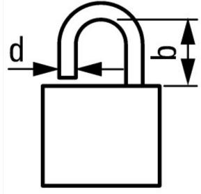
d = 4 - 8 mm  $b + d \le 47 \text{ mm}$  d = 0.16 - 0.31 d = 4 - 8 mm d = 4 - 8 mm
