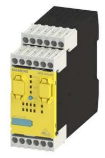
SIRIUS, Central unit 3RK3 ASIsafe Extended for modular Safety system 3RK3 2/4 F-DI, 4 DI, 1 F-RO, 1 F-DO,24 V DC Monitoring of ASI slaves Control of 10 safe outputs on AS-Interface bus parameterizable using software Safety ES 45 mm width screw terminal Up to SIL3 (IEC 61508) Up to Performance Level E (ISO 13849-1) 2 extension modules connectable
