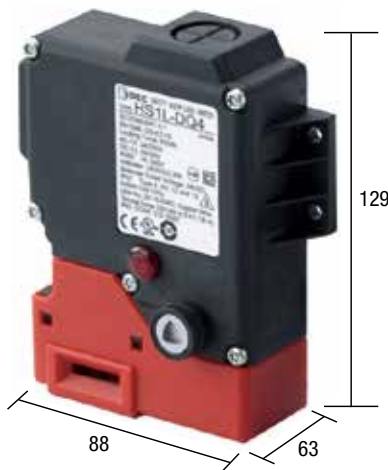
Conventional (HS1L): Volume 715 cm 3 Locking force 3000N
