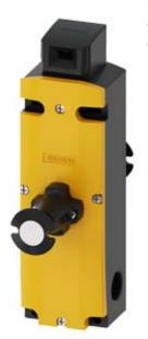
Safety position switch with tumbler Locking force 1300 N 5 directions of approaches Spring-locked Emergency release at the rear and Escape release on the front Magnet voltage 24 V DC Monitoring actuator 2 NC/1 NO Monitoring magnet 2 NC/1 NO Supplied without actuator. Actuator 3SE5000-0AV0. please order separately
