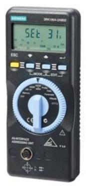
AS-Interface Addressing unit V3.0 for setting the addresses of AS-i slave modules Input/output test and further functions AS-i specification V3.0 M12 connection socket with addressing cable 1.5 m (M12 connector/hollow plug) with batteries (4 x 1.5 V LR6) Addressing of user modules via accessory 3RK1901-1MA00
