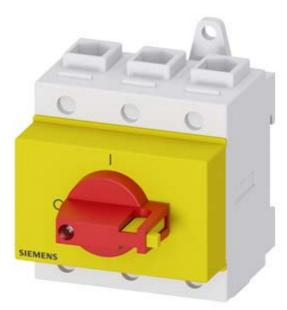
SENTRON, Switch disconnector 3LD, emergency switching-off switch, 3- pole, lu: 100 A, operating power / at AC-23 A 400 V: 37 kW, installation in distribution boards, knob-operated mechanism, Red / yellow, handle direct at the switch
