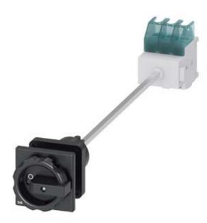
SENTRON, Switch disconnector 3LD, main switch, 3-pole, Iu: 32 A, Operating power / at AC-23 A at 400 V: 11.5 kW, floor mounting with door coupling, rotary operating mechanism, black, central mounting 22.5 mm of the handle
