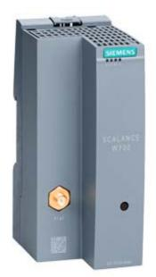
IWLAN Access Point, SCALANCE W761-1 RJ45, 1 radio, 1 R-SMA antenna port, IEEE 802.11a/b/g/h/n, 2.4/5GHz, gross data rate 150 Mbit/s, 1x RJ45 max. 100 Mbit/s, 24 V DC, terminal block, IP20, 0... +55°C, WPA2/802.11i/e, observe national approvals! CERT ID: ELN-W1-RJ-E1, scope of delivery: Manuals on CD-ROM German/English, 1x terminal block; for operation outside of USA/Israel
