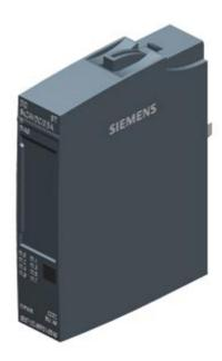
SIMATIC ET 200SP, Digital output module, DQ 8x 24V DC/0,5A Standard, Source output (PNP,P-switching) Packing unit: 1 piece, fits to BU-type A0, Colour Code CC02, substitute value output, module diagnostics for: short-circuit to L+ and ground, wire break, supply voltage
