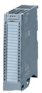
SIMATIC S7-1500 analog input module AI 8xU/R/RTD/TC HF, 16 bit resolution, up to 21 bit Resolution at RT and TC, accuracy 0.1%, 8 channels in groups of 1; common mode voltage: 30 V AC/60 V DC, Diagnostics; Hardware interrupts Scalable temperature measuring range, thermocouple type C, Calibrate in RUN; Delivery including infeed element, shield bracket and shield terminal: Front connector (screw terminals or push-in) to be ordered separately
