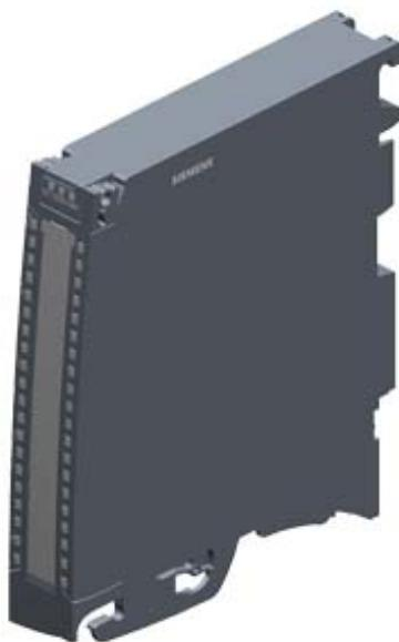
SIMATIC S7-1500 Analog input module AI 4xU/I/RTD/TC ST, 16 bit resolution, Accuracy 0.3%, 4 channels in groups of 4; 2 channels for RTD measurement; Common mode voltage 10 V; Diagnostics; Hardware interrupts; Delivery including push-in front connector, infeed element, shield bracket, and shield terminal
