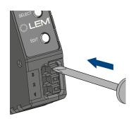
To remove wiring easily, use any tools or a 2.5 mm flat screwdriver
