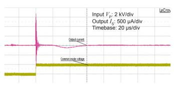
Figure 12: Detail of typical common mode perturbation (2000 V step with 6 kV/μs,  $R_{M}$  = 100 Ω)
