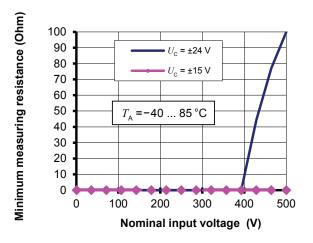
Figure 2: Minimum measuring resistance For  $T_{\rm A}$  under 80 °C, the minimum measuring resistance is 0  $\Omega$  whatever  $U_{\rm C}$
