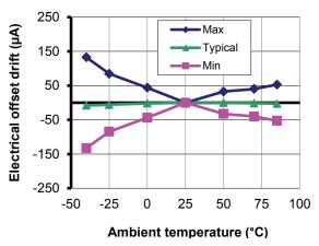
Figure 3: Electrical offset thermal drift
