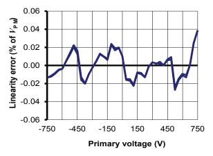
Figure 15: Typical linearity error at 25 °C
