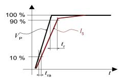
Figure 17: Response time  $t_r$  and reaction time  $t_{ra}$
