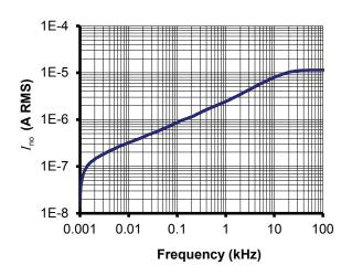
Figure 14: Typical total output RMS noise current with  $R_{\rm M}$  = 50  $\Omega$  $(f_c$  is upper cut-off frequency of bandpass, low cut off frequency is 1 Hz)
