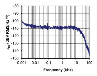
Figure 13: Typical output RMS noise voltage spectral density  $e_{\rm no}$  with  $R_{\rm M}$  = 50  $\Omega$
