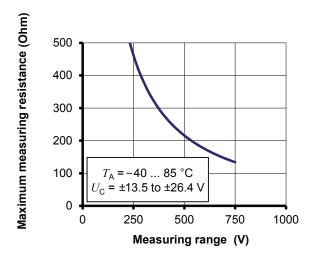
Figure 1: Maximum measuring resistance
