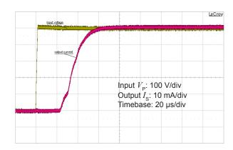
Figure 6: Typical step response (0 to 500 V)
