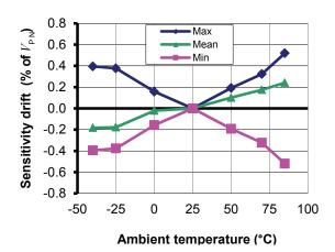
Figure 5: Sensitivity thermal drift
