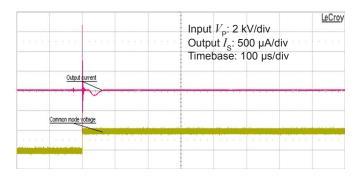
Figure 11: Typical common mode perturbation (2000 V step with 6 kV/ $\mu$ s  $R_{\rm M}$  = 100  $\Omega$ )
