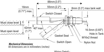
Wiring Detail:-Red = Switch Green = Thermistor
