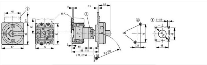
Shaft and interlock extension with ZAV-P3 + ZVV-P3 possible; max. 4 x 25 = 100 mm
