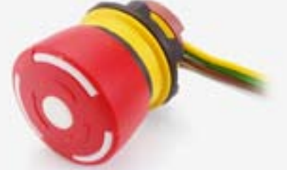
Emergency-stop non illuminated, ribbon cable, twist release, 32 mm diameter for 22.5 mm mounting, foolproof to EN 60947-5-5
