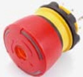
Emergency-stop red LED illuminated, plug-in terminals, twist release, 32 mm diameter for 22.5 mm mounting, foolproof to EN 60947-5-5
