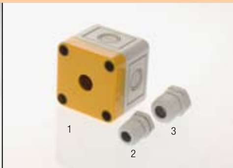
Emergency-stop switch enclosure with 22.5 mm Ø mounting hole, 65 mm (w) x 65 mm (h) x 57 mm (d), anti twist hole. Cable gland M16 or M20, IP66
