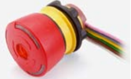
Emergency-stop red LED illuminated, ribbon cable, twist release, 32 mm diameter for 22.5 mm mounting, foolproof to EN 60947-5-5
