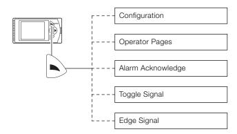
Fig. 6: Programmable soft key
