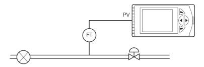
Fig. 12: Single PV with totalization
