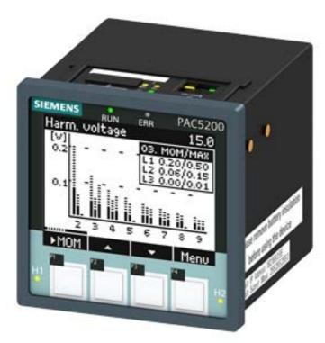
SENTRON, measuring device and power quality recorder, 7KM PAC5200, LCD, L-L: 690 V, L-N: 400 V, MODBUS TCP, apparent / active / reactive energy / cos phi, harmonics: 2nd - 40th, THD, Cl. 0.5 acc. to IEC61557- 12 or Cl. 0.5S acc. to IEC62053-22
