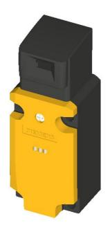
SAFETY POS. SWITCH W. SEPARATE ACTUATOR, METAL HOUSING, 40MM, 1X(M20X1.5) SLOW-ACTION CONTACTS 2NC/1NO; W. 2 LEDS, 24V DC YELLOW/GREEN, 5 DIRECTIONS OF APPROACH
