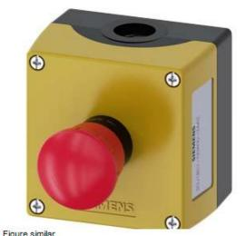
ENCLOSURE FOR COMMAND DEVICES, 22MM, ROUND, ENCLOSURE MATERIAL PLASTIC, ENCLOSURE TOP PART YELLOW, 1 COMMAND POINT PLASTIC, COMMAND POINT AT CENTER, A=EM. STOP MUSH. PUSHB. RED, 40MM, ROTATE TO UNLATCH, 1NC, SCREW TERMINAL, BASE MOUNTING,
