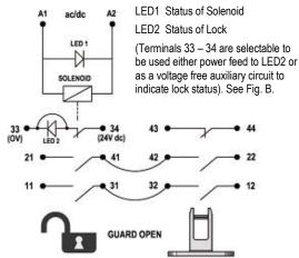
The connections between terminals 31/32 and 41/42 are made using wire links inside the switch (factory fitted). These links are able to be removed at installation to allow individual monitoring of the lock status and tongue status.
