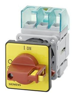
MAIN/EMERG. STOP SWITCH 3-POLE IU=16, P/AC-23A AT 400V=7.5KW FRONT MOUNTING FOUR-HOLE MOUNTING KNOB-OPERATED MECHANISM RED/ YELLOW (EMERG. STOP)
