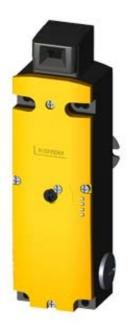
SAFETY POSITION SWITCHES WITH SOLENOID INTERLOCKING LOCK. FORCE 2600N,5 APPR. DIR. METAL HOUSING,3X(M20X1.5) SPRING-LOCKED, ESCAPE RELEASE FROM REAR AND AUX. RELEASE ON FRONT MAGNET VOLTAGE 24V DC, MONITOR. OF ACTUATOR 2NC/1NO, MONITOR. OF MAGNET 2NC/1NO LEDS YELLOW/GREEN
