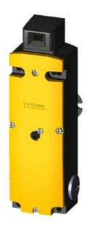
SAFETY POSITION SWITCHES WITH SOLENOID INTERLOCKING LOCK. FORCE 2600N,5 APPR. DIR. METAL HOUSING,3X(M20X1.5) SPRING-LOCKED, ESCAPE RELEASE FROM REAR AND AUX. RELEASE ON FRONT MAGNET VOLTAGE 24V DC, MONITOR. OF ACTUATOR 2NC/1NO, MONITOR. OF MAGNET 2NC/1NO
