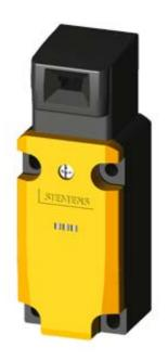
SAFETY POS. SWITCH W. SEPARATE ACTUATOR, METAL HOUSING, 40MM, 1X(M20X1.5) SLOW-ACTION CONTACTS 2NC/1NO; W. 2 LEDS 230V AC YELLOW/GREEN, 5 DIRECTIONS OF APPROACH
