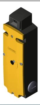
SAFETY POSITION SWITCHES WITH SOLENOID INTERLOCKING LOCK. FORCE 2600N,5 APPR. DIR. METAL HOUSING,3X(M20X1.5) SPRING-LOCKED, AUXILIARY RELEASE ON FRONT MAGNET VOLTAGE 230V AC, MONITOR. OF ACTUATOR 2NC/1NO, MONITOR. OF MAGNET 2NC/1NO
