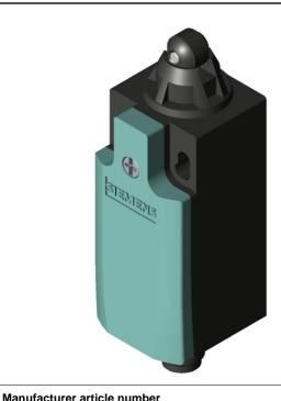
SIRIUS POSITION SWITCH; PLASTIC HOUSING ACC. TO EN50047, 31MM 1NO/1NC SNAP-ACTION CONTACTS INTEGRATED (NOT REPLACEABLE) W. M12 CONNECTOR, 4-POLE PIN ASSIGNMENT: PIN1=21, PIN2=22, PIN3=13,PIN4=14, FOR MAX.250V AND 4A ROLLER PLUNGER W. PLASTIC ROLLER 10MM
