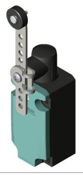
SIRIUS POSITION SWITCH METAL ENCLOSURE 40MM TO EN50041 DEVICE CONNECTION 1X (M20X1.5) 1NO/ 2NC SNAP-ACTION CONTACTS ROTARY ACTUATOR RIGHT/LEFT ADJUSTABLE,
