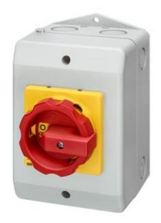
EMERG. STOP SWITCH 3-POLE IU=16, P/AC-23A AT 400V=7.5KW 1 N-TERMINAL + 1 PE-TERMINAL INSULATION-ENCLOSED, IP65 ROTARY ACTUATOR RED/YELLOW (EMERG. STOP)
